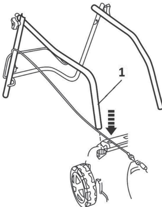
Attach the upper part of the handle to the lower part of the handle using the supplied screws with wing nuts (see the following figure).
