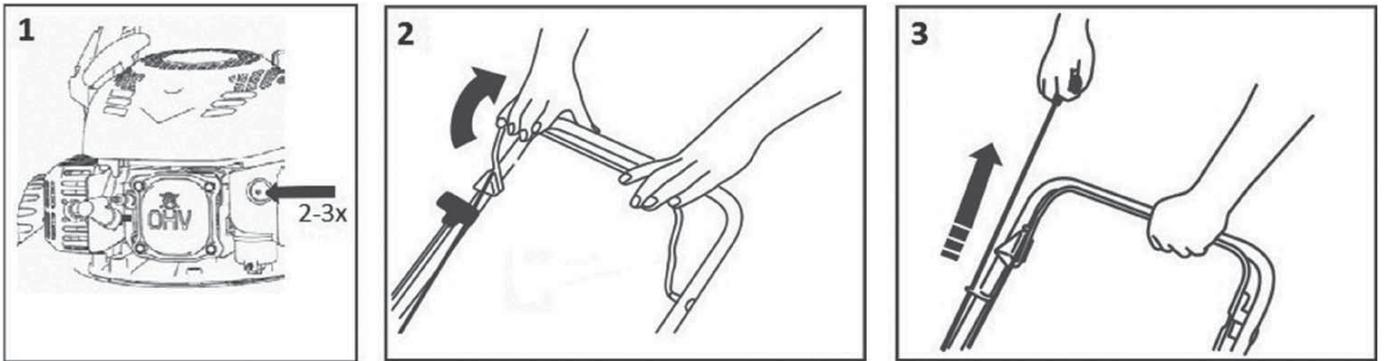
Pull the start/brake lever to the handle and hold it, then pull the pull cord. The engine should start after 3-4 pulls.
