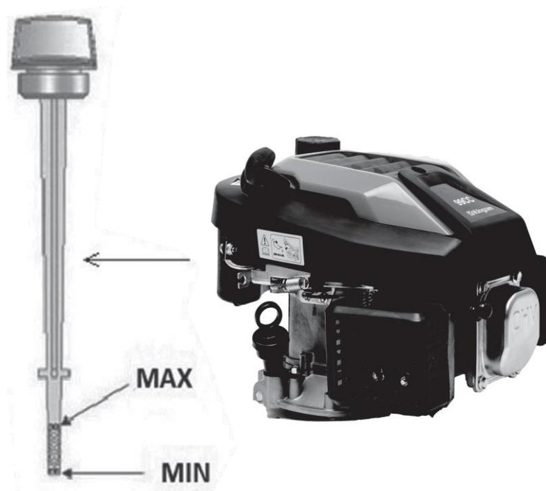
The device is supplied **without engine oil**. Before the first start-up, fill engine oil SAE30 or 15W-40 (approx. 600 ml) according to the following instructions:
